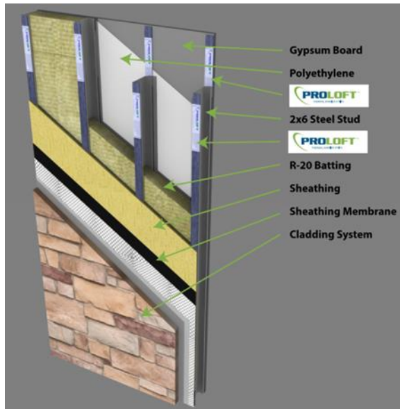
Figure 1: Typical Steel Stud Wall Assembly
